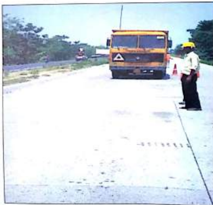
Fig. 40 Load testing of instrumented pavement
