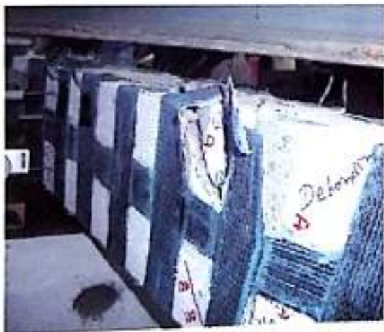
Fig. 63 (a-b) Crushing failure of concrete and debonding of CFRP fabric strips of PTT-1
