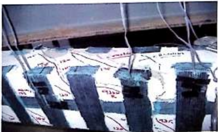
Fig. 63 (a-b) Crushing failure of concrete and debonding of CFRP fabric strips of PTT-1
