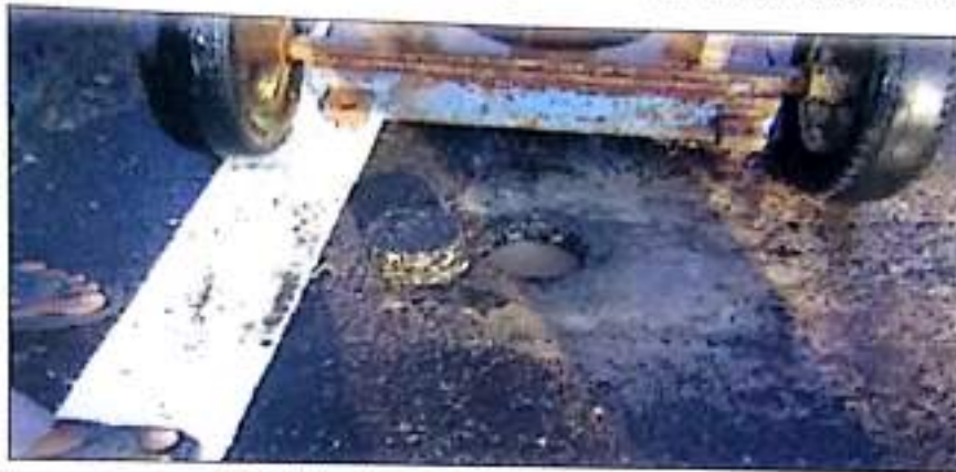
Fig. 13 Bituminous cores from experimental test track
