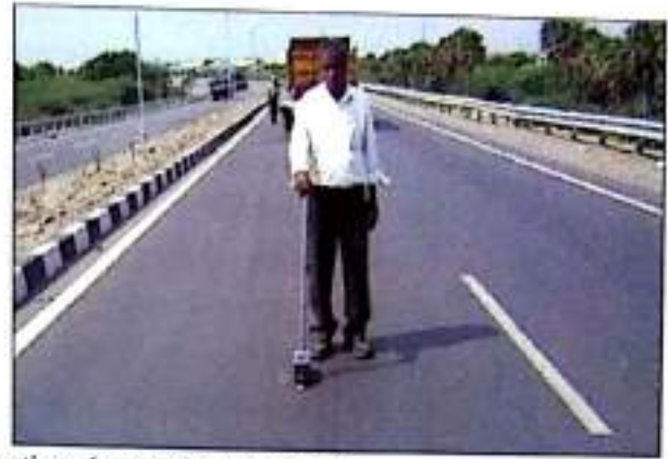
Fig. 12 Deflection and roughness observations of copper slag embankment
