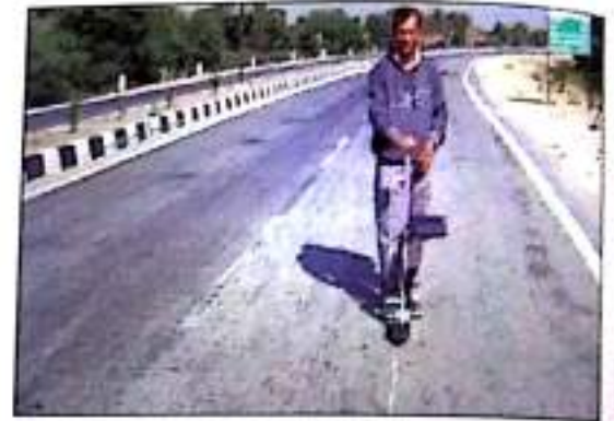
Fig. 16 Deflection measurement by using Benkelman beam
