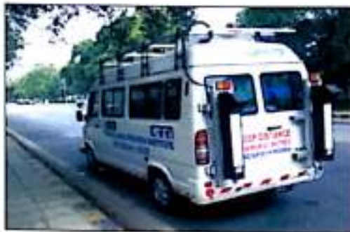
Fig. 53 Automated road survey system for measurement of pavement surface roughness
