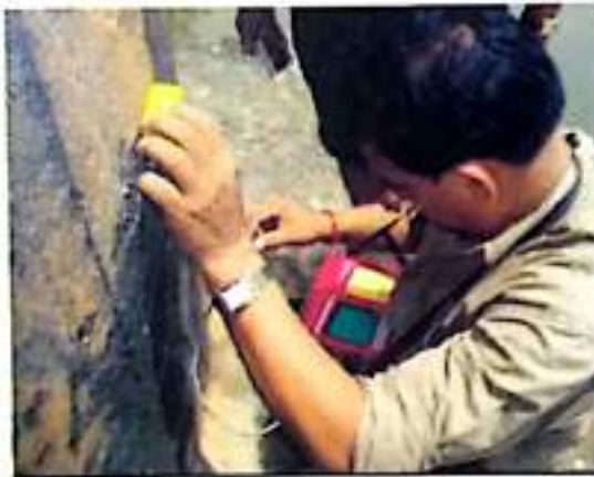
(a) Concrete cover testing
