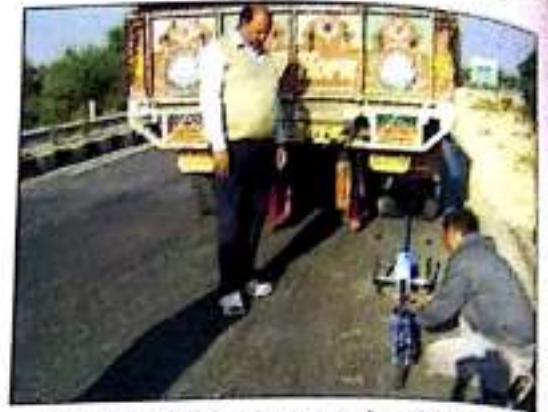
Fig. 15 Roughness measurement by using dipstick
