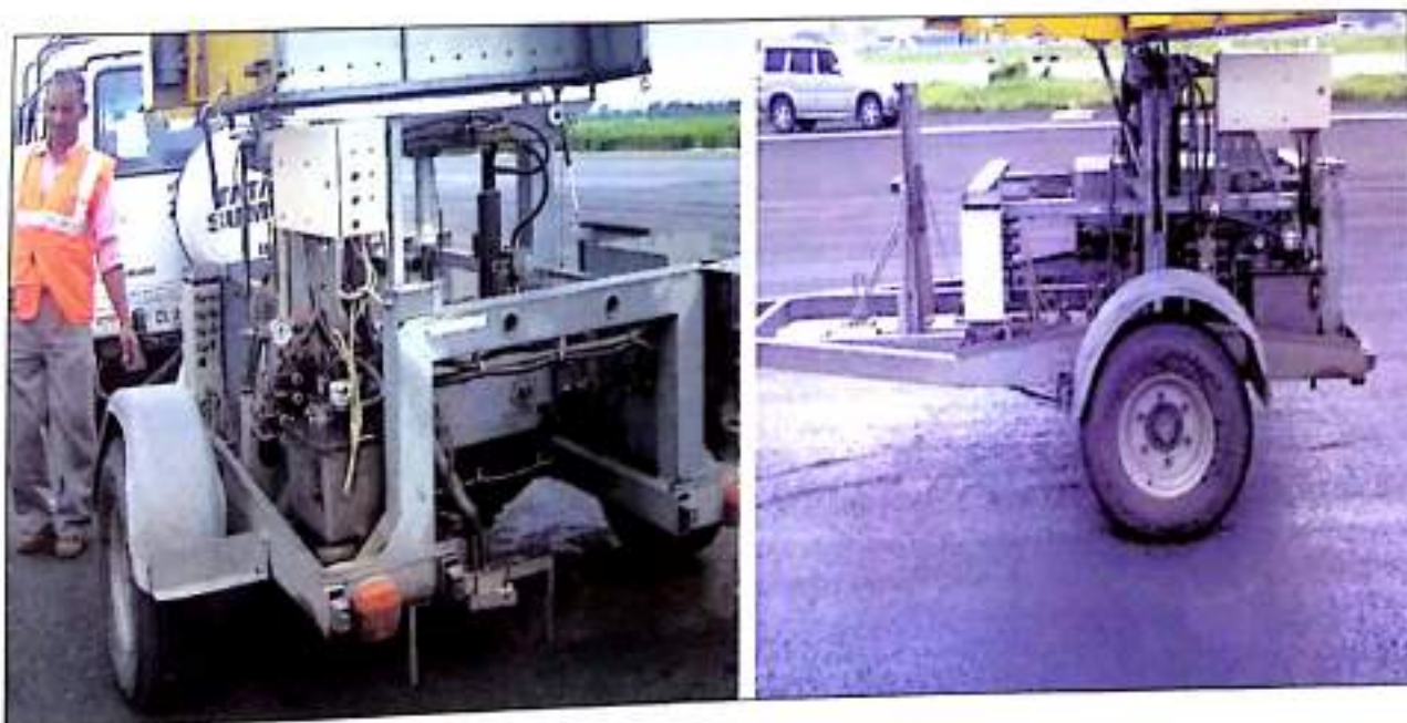
Fig. 58 FWD deflection measurements on the airfield pavement
