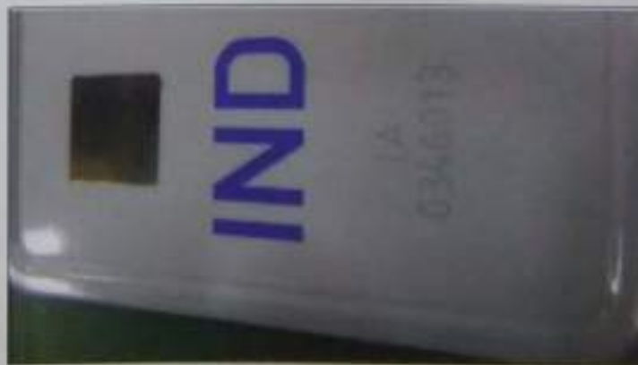
Fig. 114 A view of laser code number and other security features of HSRP
