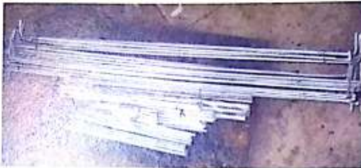
(a) Hot dipped galvanized bars
