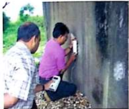
(b) Concrete resistivity test
