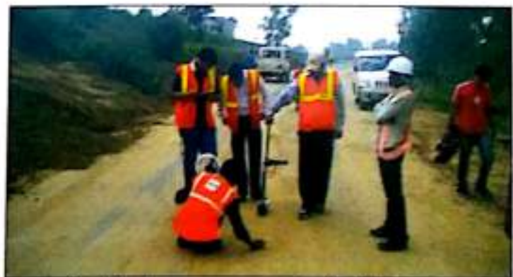
Fig. 33 Roughness measurements using Dipstick in progress on reach 3 on NH-1
