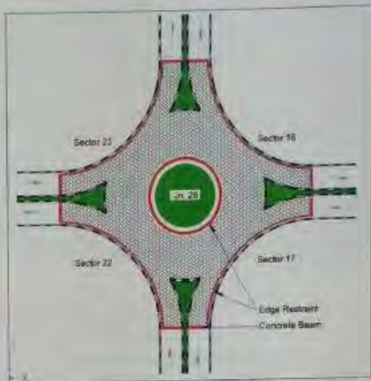
Fig. 73 Typical laying pattern of concrete paver blocks at Rotary Jn. 26.
