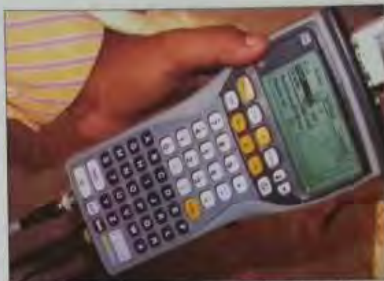
Fig. 91 Testing of corrosion of rebar embedded in concrete slab specimen with Galvapulsa
