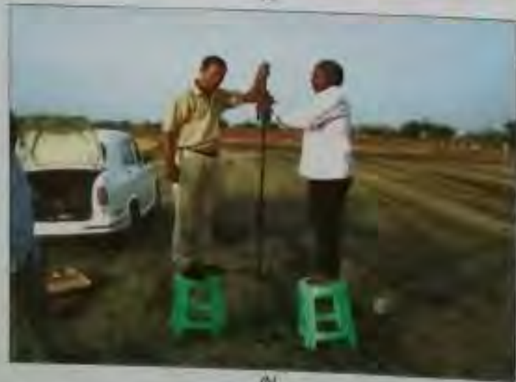
Fig. 23 (a & b) Plate load and Dynamic cone penetration tests in progress
