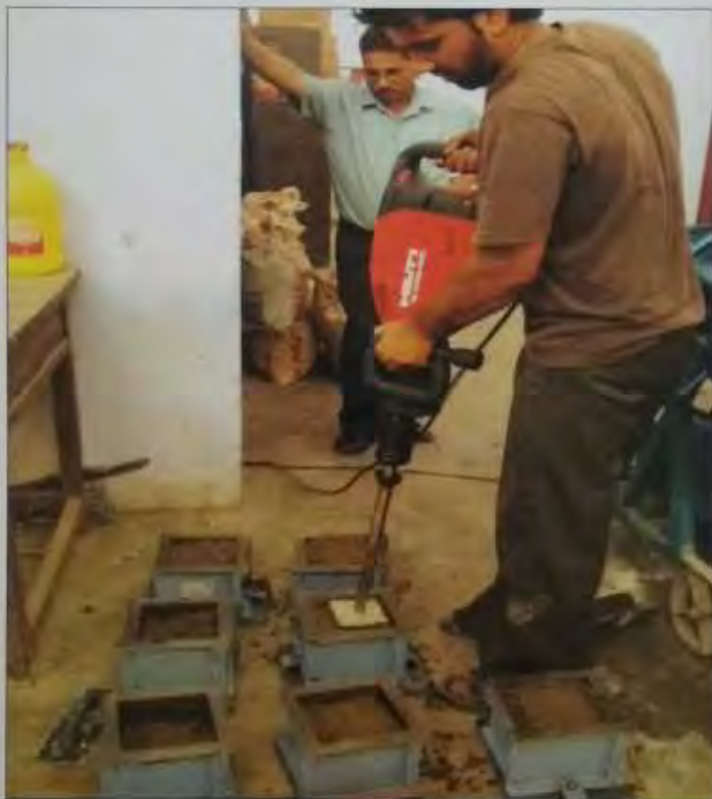
Fig. 49. DLC being compacted with the help of Jack Hammer
