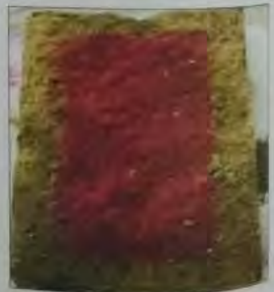
Fig. 51. CLSM specimen showing carbonation depth
