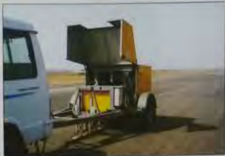
Fig. 74 Deflection measurements using FWD on runway at Surat Airport
