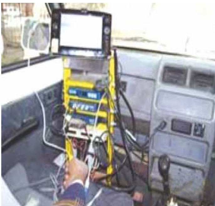
GPS based Data Acquisition System along with Fuel Flow Detector Meter and Engine RPM Meter
