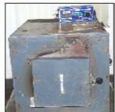
MUFFLE FURNACE, 1000°C
