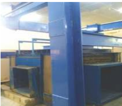
Large Scale Model Study for Underpass Intersection by Box Jacking with Soil Nailing
