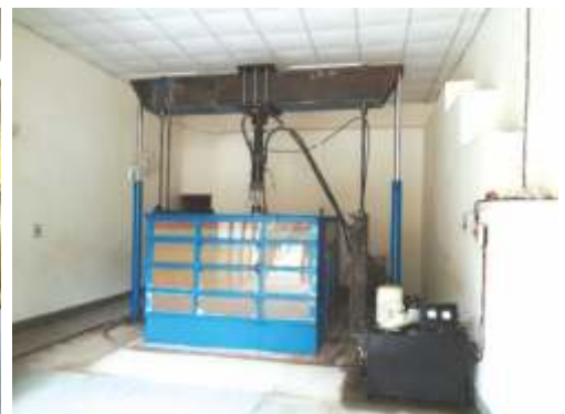
Large Scale Cyclic Plate Load Test Facility
