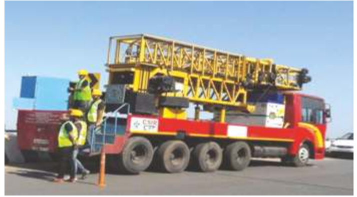
Mobile Bridge Inspection Unit
