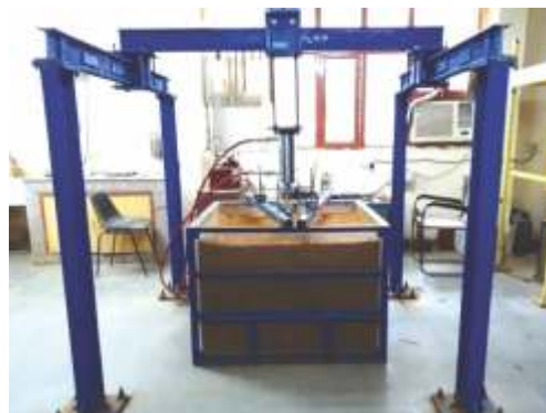
Physical model testing (Static loading) facility for embankments and foundations
