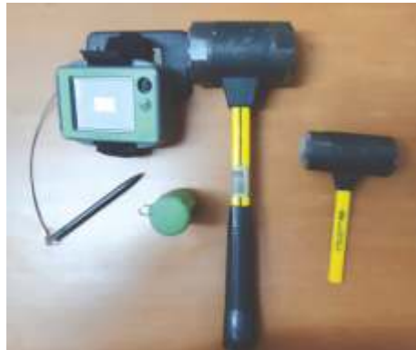
Pile Integrity Test Apparatus
